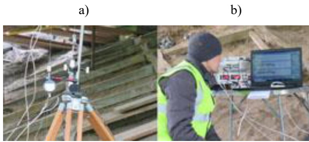
Fig. 6. Views of the installation of a potentiometric linear displacement sensor and a digital clock-type indicator under beam B-10 (a) and an analog-to-digital converter with a computer (b)
